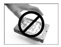
Do not touch the printed circuit board assembly with your hand or tools.
