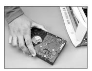
Clothing generates static electricity. Do not allow clothing to touch the hard drive or printed circuit board assembly.
