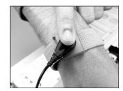
Check grounding straps daily to ensure proper functioning.
