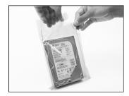
Remove the hard drive by grasping it by its sides. Do not touch the circuit boards.
