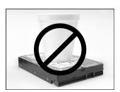
CAUTION: Western Digital hard drives install easily. Never force a hard drive into a bay, hammer on the hard drive, or touch its printed circuit board assembly. Use caution when installing data and power connectors to avoid damaging pins. Double-check that all cables are properly connected.
