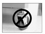
Always use stationary racks or benches. When a system is on, avoid bumping or moving the test racks. This can cause head media damage.
