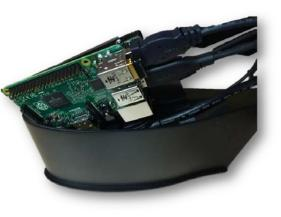
Step 9: Plug in USB power cable to a 5V, 2A adapter
