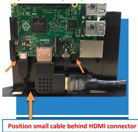
**Step 4:** Bend the PiDrive Cable to form a curve. This will help it fit in the enclosure.
