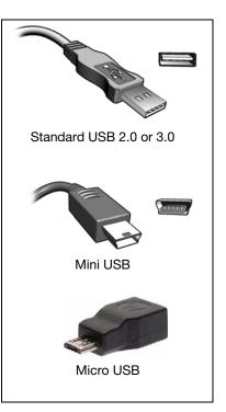
**USB 3.0.** USB 3.0 transfers data at a maximum rate of 4.80 Gb/s. Sustained data transfer rates, usually from 100 to 300 MB/s, vary depending on many factors, including the type of device, data being transferred, and computer system speed.
