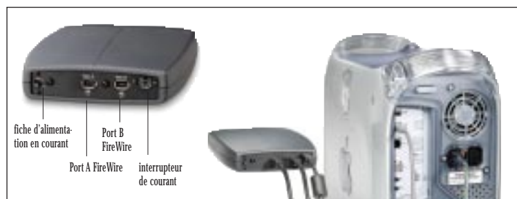
Installation du disque dur Western Digital FireWire
